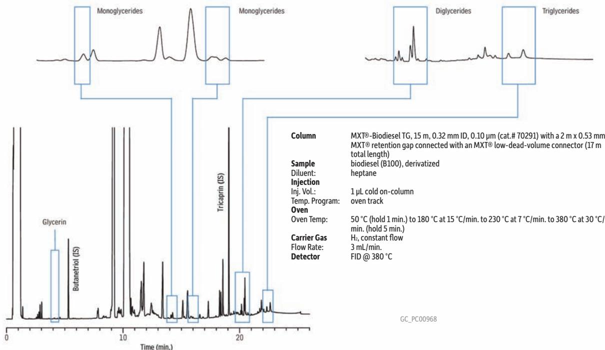
**Figure 5** Excellent chromatographic quality and resolution on the 0.53 mm MXT®-Biodiesel TG column with the Integra-Gap® integrated retention gap.
