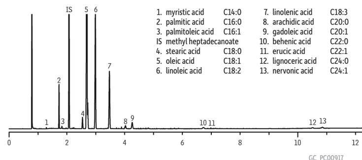
Column: Stabilwax®, 30 m, 0.32 mm ID, 0.25 µm (cat. # 10624)
