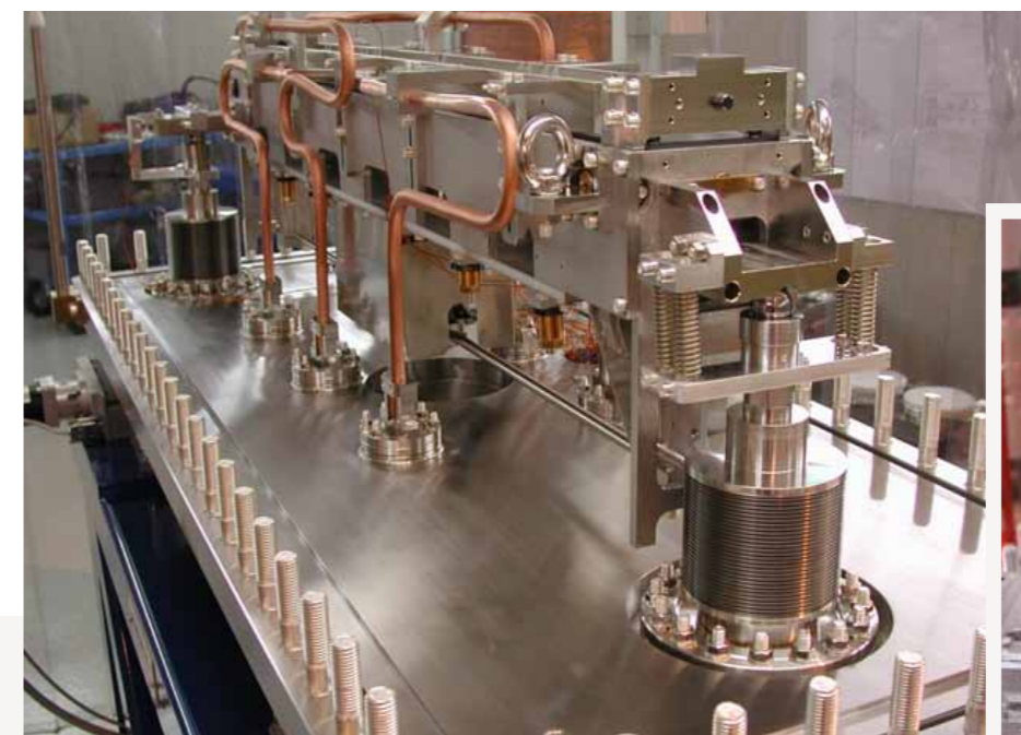
■ Mirror Chamber for Protein Crystallography Beamline (M1) X06DA Swiss Light Source SLS Villigen (Switzerland)
