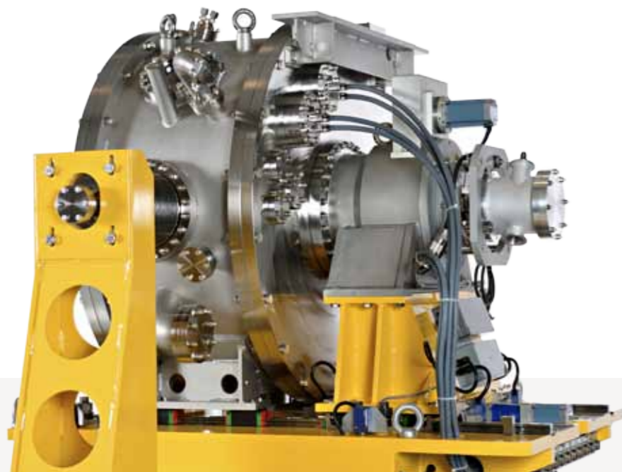
■ Fixed exit double channel DCM Monochromator (2.5 ÷ 100 keV) for ID06 Beamline European Synchrotron Radiation Facility - ESRF- Grenoble (France)
