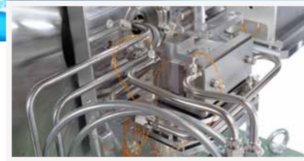
■ Fixed exit double channel DCM Monochromator (3.5 ÷ 25 keV) for BL-1A Beamline Photon Factory KEK Tsukuba (Japan)
