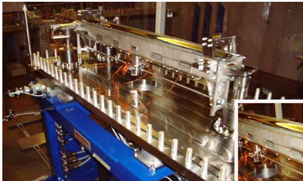
■ Mirror Chamber for Protein Crystallography Beamline (M2) X06DA Swiss Light Source SLS Villigen (Switzerland)
