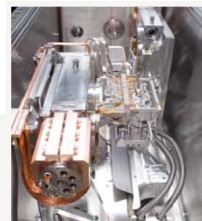
■ Double Crystal/Multilayer Monochromator (energy range ~ 8 ÷ 45 keV) for TOMCAT Beamline Swiss Light Source SLS Villigen (Switzerland)
