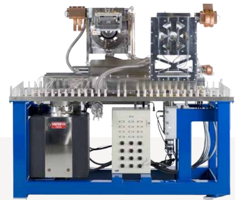
■ Double Crystal/Multilayer Monochromator (energy range ~ 8 ÷ 45 keV) for TOMCAT Beamline Swiss Light Source SLS Villigen (Switzerland)
